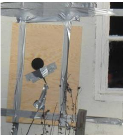
Figure 4 - Microphone in contact with the measurement plate was not in case for the examined cases. The measurement plate was less than one (1) square meter.
