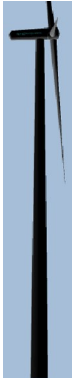
Figure 11 - WTG SWT2,3-101 with nacelle 99,5 m and tower diameter 2,4 – 4,5 m, turbine blade 3,5 m from c/c tower and back side nacelle 7,0 m from c/c tower.
