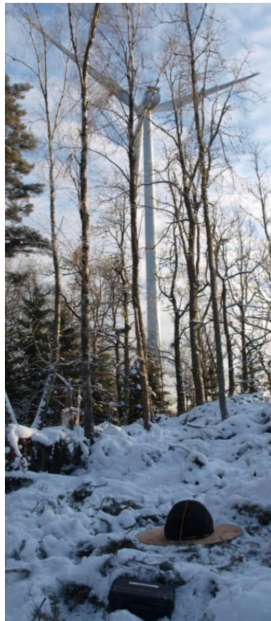
Figure 2 - Cylindrical protections and snow, with noise dampening, and with the measurement plate in slope from the microphone giving lower noise reflection.
